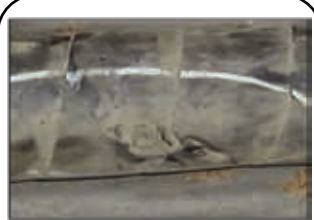
Hole in hose cover that exposes reinforcement
